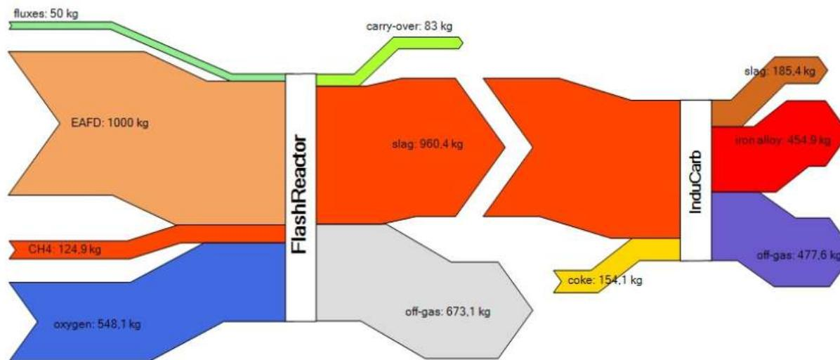
Mass balance for the treatment of 1 t of EAFD with the combined Flash Reactor – ICBR process
