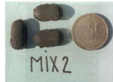
Figure 3.5 Briquettes produced with the roll compactor
