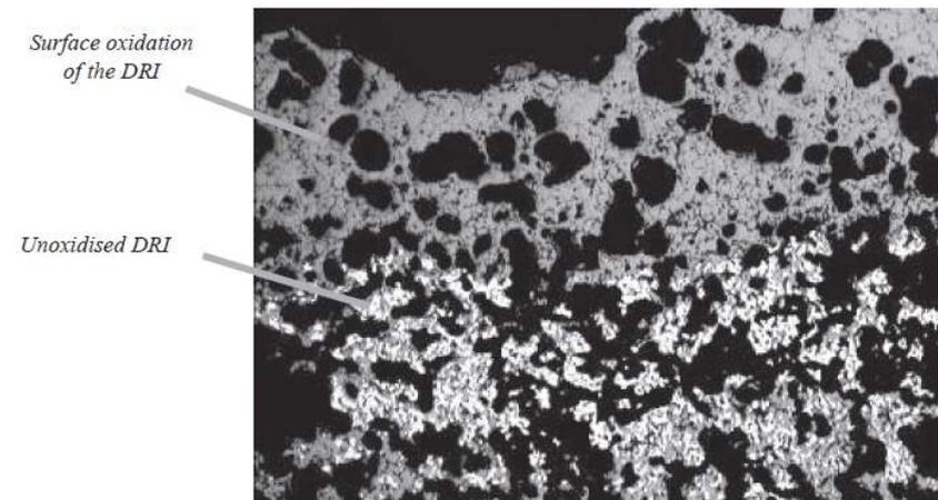
Figure 4 – Surface oxidation of the DRI produced during set-up trials
